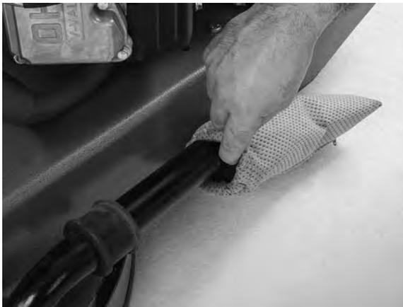
1. Remove the dust bag by working the elastic over the lip of the rubber grommet and pulling toward the rear of the machine.
