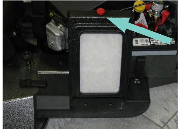
2. To reinstall the filter, correctly place the filter back in the filter retainer. Insert the bottom edge of the filter retainer against the metal guide on the bottom of the mounting area. Compress the filter retainer inward and downward to align the hole at the top of the retainer. Install the thumb screw and tighten until the filter is secured.
