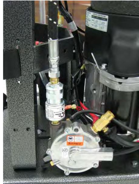
5. If a leak is detected, turn off the LP cylinder. If the leak is in a hose, replace it. If the leak is at a fitting, loosen and clean it. Apply pipe-sealing compound and re-tighten it.
