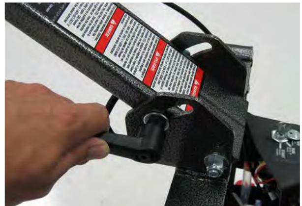
**NOTE:** The handle adjustment lever will ratchet. Pull outward and pivot the lever in the desired direction.
