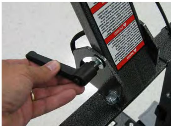
9. Adjust the handle to the desired height and tighten the handle adjustment lever.
