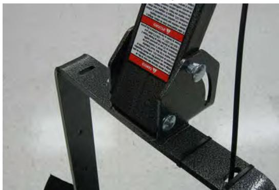
8. Place the washer and handle adjustment lever on the bolt. Thread the adjustment lever in until it is against the handle bracket, but do not tighten.
