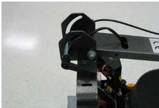
7. Rotate handle to the user position to the top of the adjustment slot. Then insert the bolt through the handle bracket and handle top.
