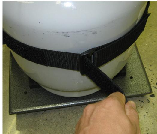
retaining strap. Remove slack by pulling on the loose end of the strap and secure back to strap.
