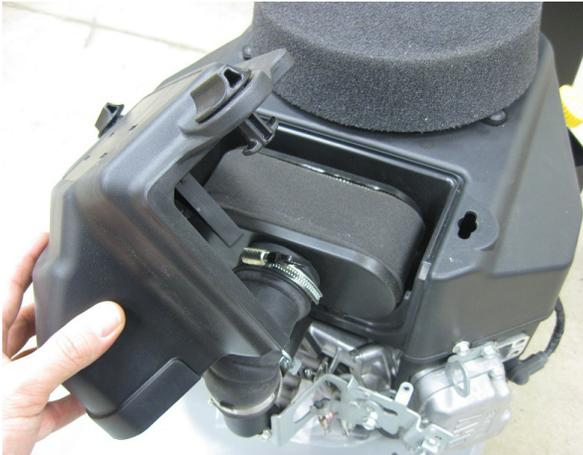
3. Turn the two knobs 1/4 turn counter-clockwise and remove the filter cover.
